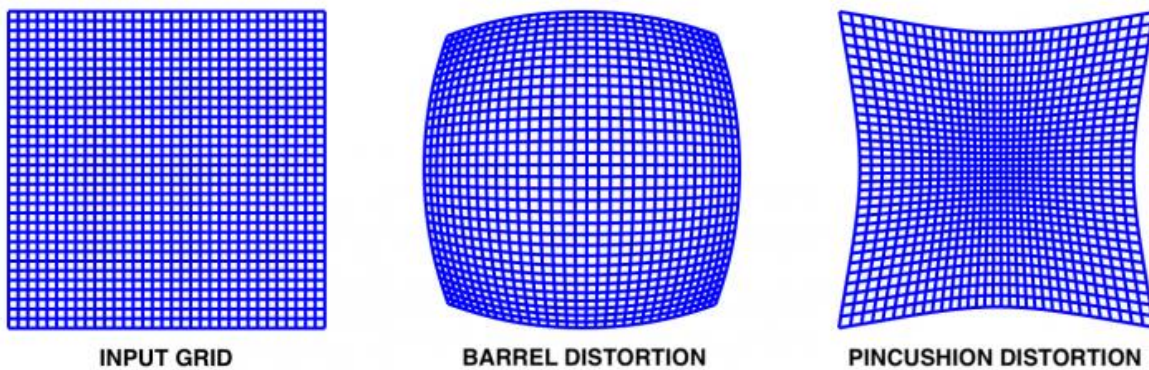
Figure: Example of the effect of barrel and pincushion distortion on a square grid.
