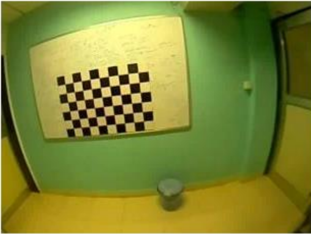
Figure: Illustration of the distortion effect. Take note of how the margins of the wall and doors are curled as a result of distortion.
